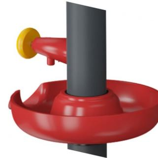
The integrated water tap open for water when pushed and stops when letting go. The water is supplied trough a pipe located inside the post with hose or pipe connection at the bottom of the post. The supply can either a loose hose or a permanent in-ground plumbing.
