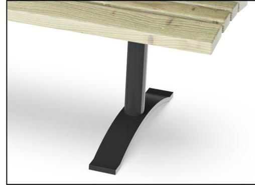
Powder coated top finish on top of galvanisation is processed in two steps: Light grinding and clean sweeping, powder coating - thickness 70-120 µm.
