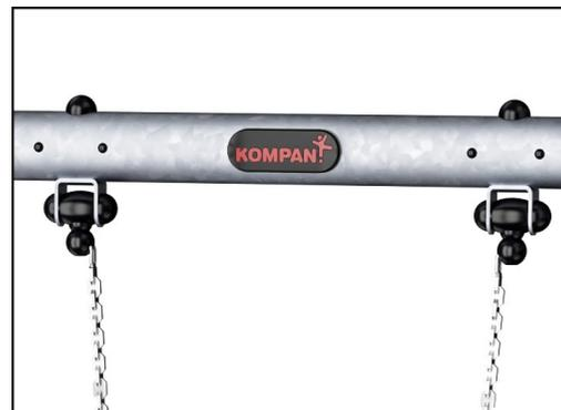
The swing hangers are made of high quality UV-stabilized nylon (PA6) housing with integrated lifetime sealed ball bearings. The height adjustable chains are fixed by a stainless steel hook with theft proof snake-eye bolt in a turn able anti twist housing. All seats with two chain fixation are available with either standard or anti-wrap suspension.
