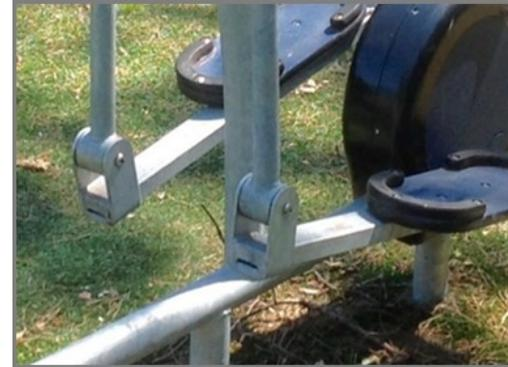
The frame and moving steel parts are constructed of hot-dip galvanized steel tube's  $\varnothing 60,3\text{mm} \times 3,2\text{mm}$ ,  $\varnothing 38\text{mm} \times 4\text{mm}$  and squared tube  $60 \times 30 \times 3\text{mm}$ . All moving connections have a stainless steel AISI 304 shaft and two ball bearings.
