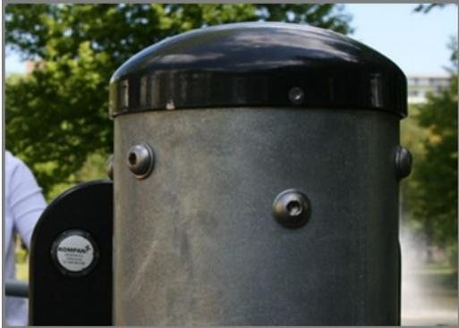
For ensuring the integrity of the main frame the support post is made of a hot-dip galvanized steel tube of  $\varnothing 159\text{mm}$ , with a wall thickness of 4mm and has a post cap made of powder-coated aluminium.
