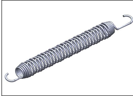
All 36 springs are made of stainless steel to ensure durability and excellent corrosion resistance. The steel wire is 3,2 mm thick and the last five windings are cone shaped to ensure long lifetime of the jumper.
