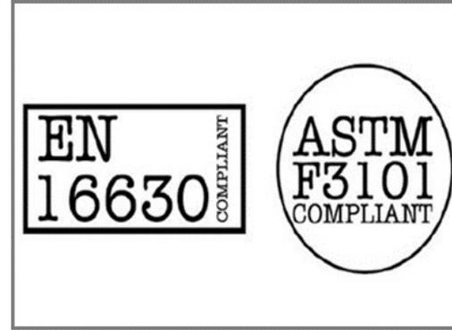
All KOMPAN fitness products are compliant with the ASTM F3101 & EN16630 Outdoor Fitness Standards. Load tests are performed as a static test by adding dynamic factors as well as safety factors to the specified load of 78kg per user. A product intended for 1 user is loaded with 420kg.
