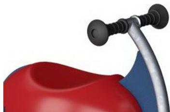
Handles are made with a molded PP insert and an outer layer of soft TPV rubber. The handles are attached to the pipe with a galvanized steel inlay to ensure strength and durability.
