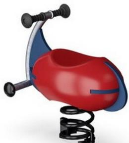
The seat is made of recyclable PE and molded in one piece with a minimum 5mm wall thickness. PE has high impact resistance across a wide temperature span which ensures vandal resistance in all locations.
